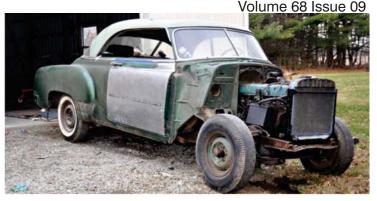
done repairs. Consequently, I had to straighten the fenders, doors, and quarter panels by hand. After all these pieces were removed, I lifted the body off the frame and attached it to the rotisserie. At that point, I removed the front and rear suspension and had the frame sandblasted and powder coated by Xtreme Powder Coating in Easton, PA.
