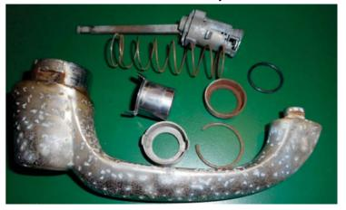
I found the engine in relatively good condition and during the disassembly, I saw that the rings were worn,
