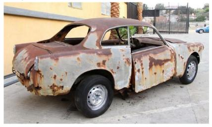
Floors are Swiss cheesed, the steering wheel rim is separating, and most fittings aside from gauges are missing. Even these are likely to be good and crusty inside.
