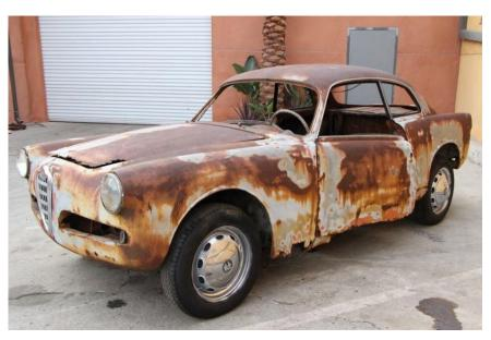
The car is so heavily corroded along the bottom that it's buckled in half aft of the doors, with apparently little more than the roof keeping it from splitting into two halves. Glass, door handles, bumpers, and much more are missing and likely gone forever.
