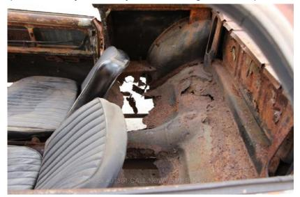
Underneath its lid, the trunk is little more than a jagged, crusty hole, but that rear axle does appear to be salvageable.
